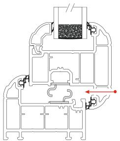
STAY GUARD ELITE SG036 on outer frame and sash for all types of stays to include Egress/Easy Clean
